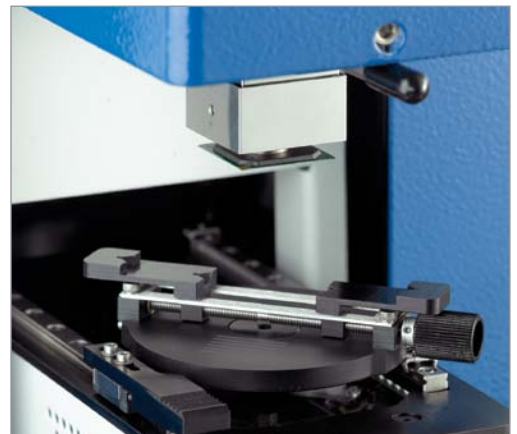
PBGA being held by Vacuum pik during Alignment procedure
