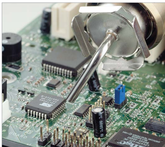
ST 300 Reflowing a PLCC
